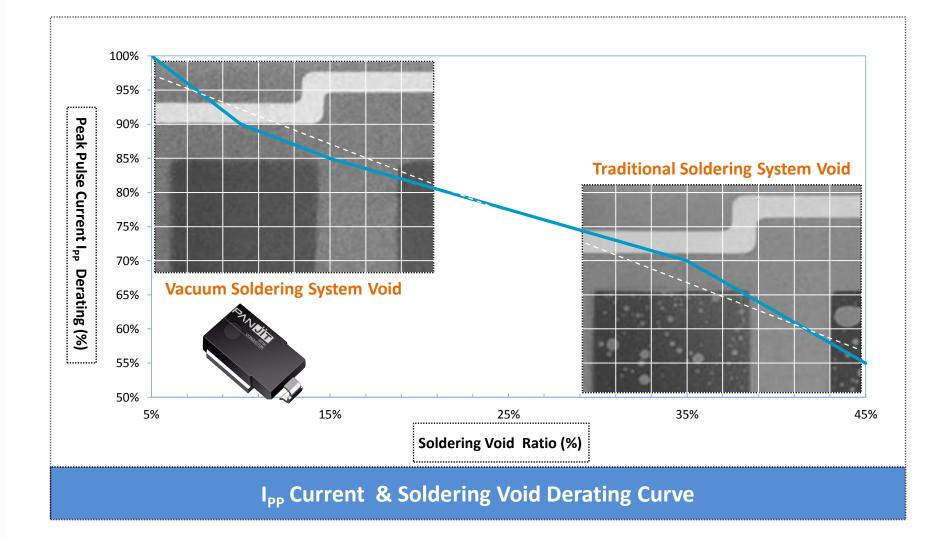
The soldering void is a key point for power TVS products, the amount of the void effects the surge current capability of the TVS
