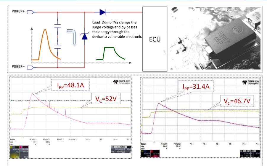
Test Rule: ISO16750-2 5a Test  $R_i=3\Omega$
