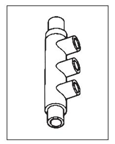
Clamping Elements — Outlet Symbols A or B, refer to socket and nut Type Z-NR, and cone Type Z cable clamping elements accommodated. These must be ordered separately.
