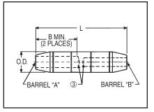
connectors are prefilled with PENETROX™. Rated up to 35 kV.
