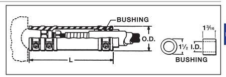
For oil filled cables a third clamp is provided to effect an oil-tight joint.
