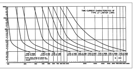
Figure 5: Current in Amperes Replaceable-link Limiters
