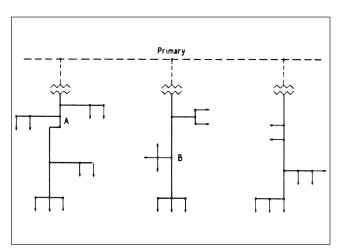
Figure 1: Radial Secondary Distribution System
