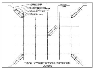
Figure 2: Typical Secondary network Equipped with Limiters
