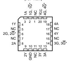
\*G on '125 and 'LS125A devices; G on 126 and 'LS126A devices NC – No internal connection
