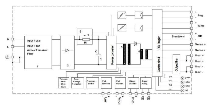
1) Active Transient Filter 2) Rectifier 3) Inrush Current Limiter 4) Load Capacitor 5) Power Transformer 6) Storage Choke Lighting: CV = constant voltage operation CC = constant current operation SD = shutdown operation OT = temperature failure >70°C
