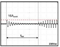
(Fig.8 inrush with an ESB)
