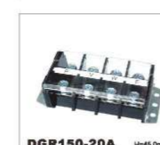
DGR150-20A H=48.0mm 1000V/155A 70mm 2 600V/155A 20-2/0AWG Poles 1P-XXP
