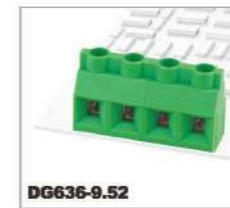
DG636-9.52 1000V/32A 0.2-4.0mm 2 300V/30A 26-10AWG Poles 2P,3P-24P
