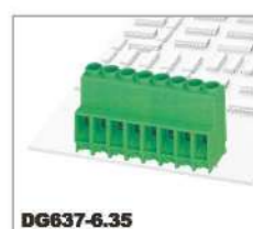
DG637-6.35 IEC 1000V/32A 4.0mm 2 600V/30A 28-10AWG Poles 1P-XXP
