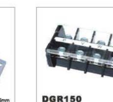
DGR150 Steel H=48.0mm 800V/155A 50mm 2 600V/155A 20-2/0AWG Poles 1P-XXP
