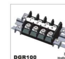
DGR100 Steel H=43.5mm 800V/100A 35mm 2 600V/101A 20-2AWG Poles 1P-XXP
