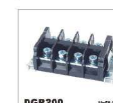
DGR200 H=58.0mm 800V/200A 95mm 2 600V/200A 20-4/0AWG Poles 1P-XXP
