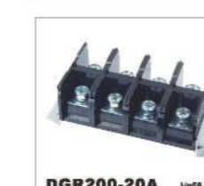
DGR200-20A H=58.0mm 800V/200A 95mm 2 600V/200A 20-4/0AWG Poles 1P-XXP
