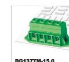
DG137TM-15.0 1000V/115A 4.0-35.0mm 2 600V/115A 20-2AWG Poles 2P,3P-9P
