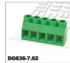
DG636-7.62 630V/32A 0.2-4.0mm 2 300V/30A 26-10AWG Poles 2P,3P-24P
