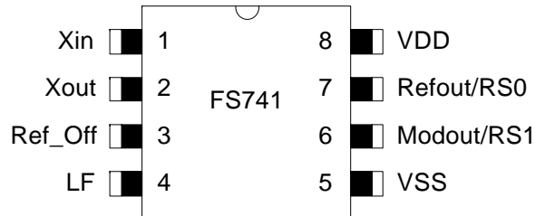
Figure 2. FS741, SOIC Package Pin Assignment
