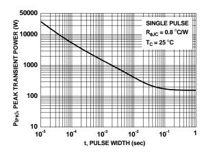
Figure 12. Single Pulse Maximum Power Dissipation
