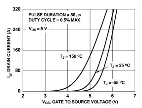
Figure 5. Transfer Characteristics
