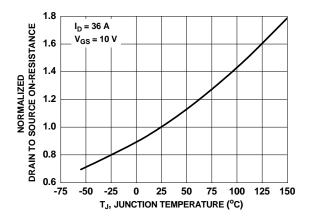
Figure 3. Normalized On-Resistance vs. Junction Temperature
