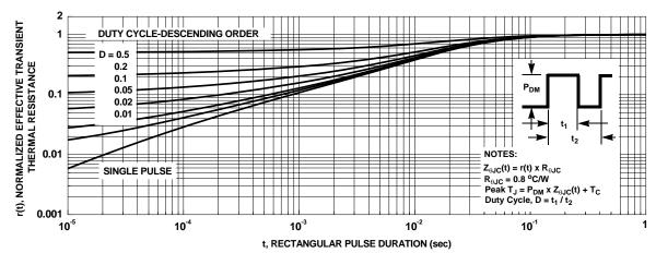
Figure 13. Junction-to-Case Transient Thermal Response Curve
