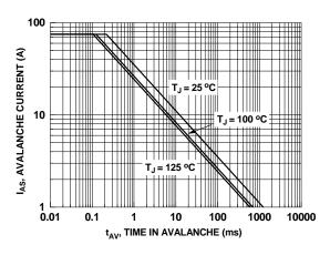
Figure 9. Unclamped Inductive Switching Capability
