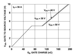
Figure 7. Gate Charge Characteristics
