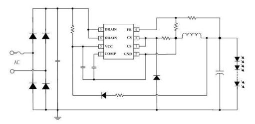
Figure 1. Typical application circuit for HW9616B
