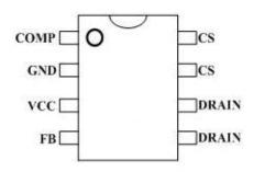
Figure 2. Pin configuration
