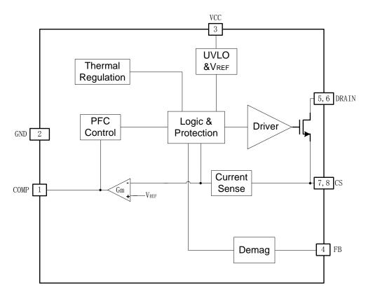
Figure 3. HW9616B Internal Block Diagram
