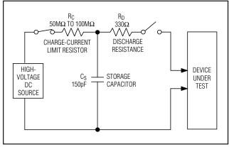
Figure 4. IEC 1000-4-2 ESD Test Model
