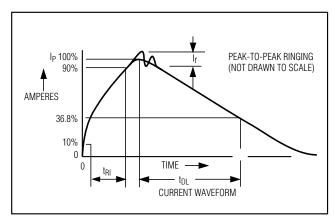
Figure 3. Human Body Model Current Waveform
