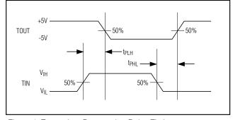
Figure 1. Transmitter Propagation-Delay Timing
