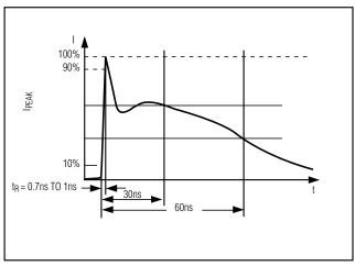
Figure 5. IEC 1000-4-2 ESD Generator Current Waveform
