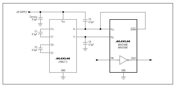
Figure 6. Powering the MAX3188E/MAX3189E
