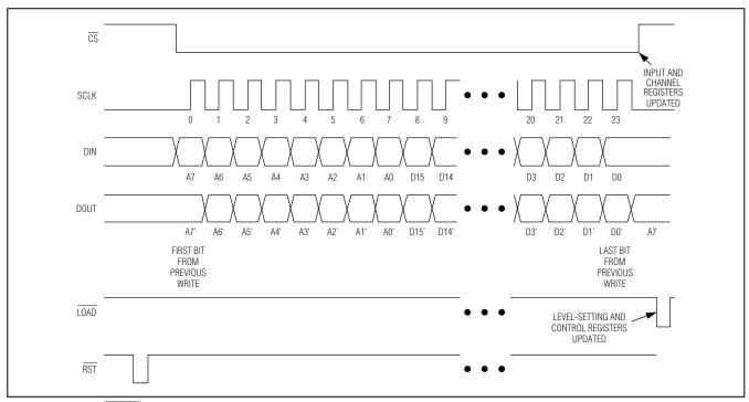
Figure 10. Using LOAD to Update the Level-Setting and Control Registers
