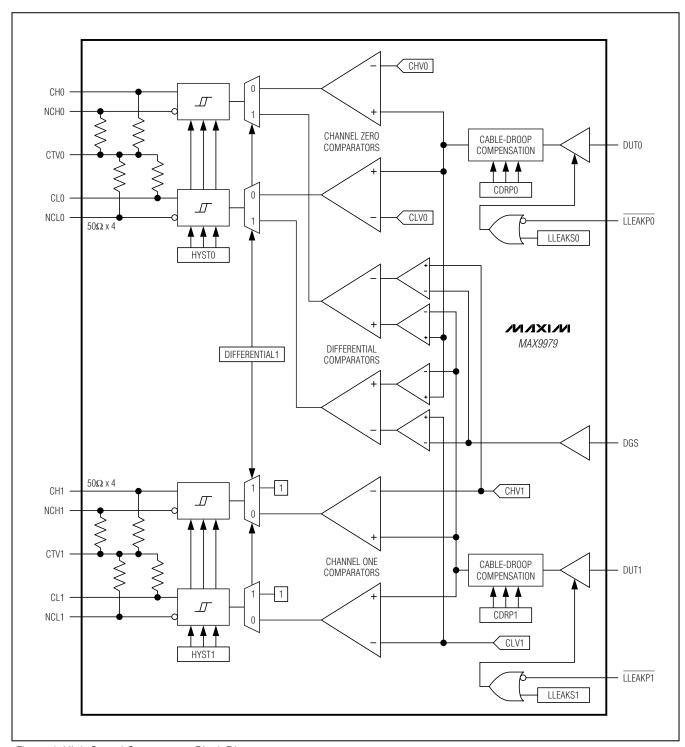
Figure 4. High-Speed Comparators Block Diagram
