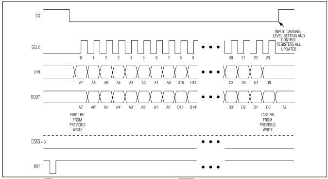
Figure 11. Using CS to Update the Level-Setting and Control Registers (LOAD Held Low)
