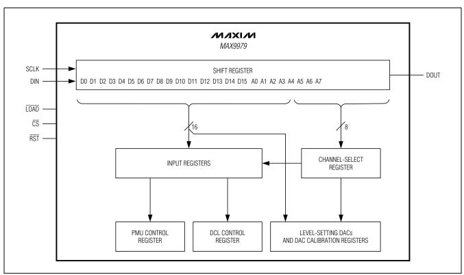
Figure 8. Serial-Interface Block Diagram
