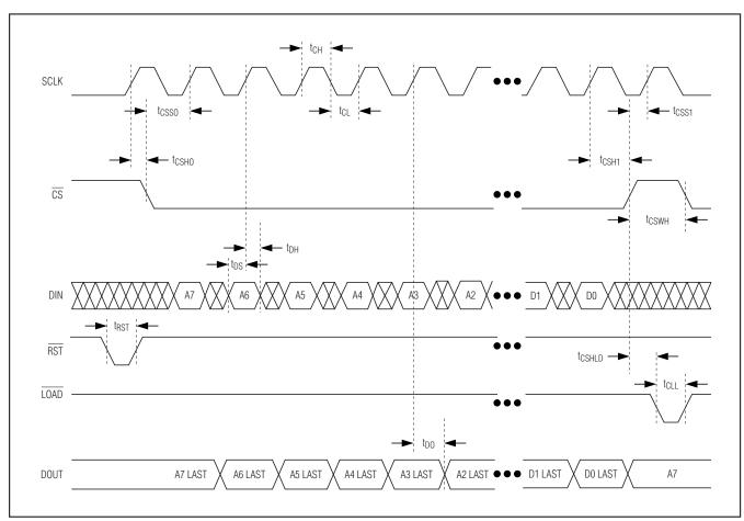
Figure 9. Serial-Interface Timing
