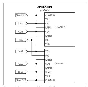
Figure 12. Arrangement of Shared DACs
