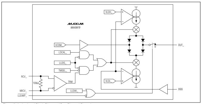
Figure 5. Active Load Block Diagram (One Channel Shown)
