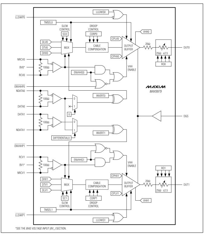
Figure 3. Driver Block Diagram
