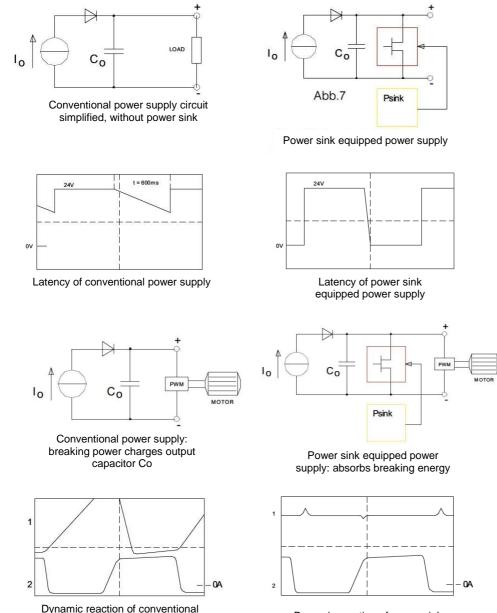
Dynamic reaction of power sink equipped power supply: load current switches between positive and negative
