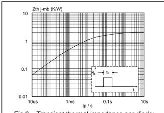
Fig.6. Transient thermal impedance per diode;  $Z_{th j\text{-}mb} = f(t_p)$ .
