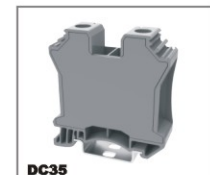
DC35 CE 1000V/125A 2.5-50mm 2 UL 600V/150A 14-1/0AWG T/W/End plate 16/55.4/-mm
