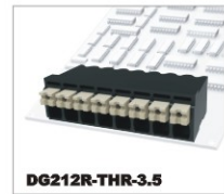
DG212R-THR-3.5 320V/17.5A 0.2-1.5mm 2 300V/12A 28-14AWG Poles 2P-24P
