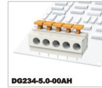
DG234-5.0-00AH 320V/10A 0.2-1.5 STR 300V/10A 30-16AWG Poles 2P-24P
