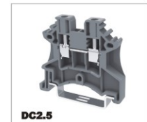
DC2.5 CE 800V/24A 0.2-4mm 2 UL 600V/25A 26-12AWG T/W/End plate 5.1/44.5/1.5mm
