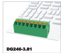
DG246-3.81 160V/9A 0.2-1.0mm 2 300V/10A 24-16AWG Poles 2P-24P
