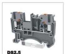
DS2.5 CE 800V/24A 0.2-4mm 2 UL 600V/20A 26-12AWG T/W/End plate 5.2/48.5/1.5mm
