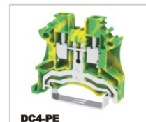
DC4-PE CE — 0.2-6mm 2 UL — 22-10AWG T/W/End plate 6.1/44.5/1.5mm
