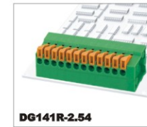
DG141R-2.54 130V/6A 0.2-1.0mm 2 150V/2A 24-20AWG Poles 1P-XXP
