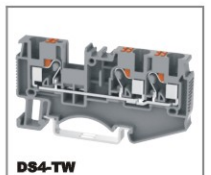
DS4-TW CE 800V/32A 0.2-6mm 2 UL 600V/30A 24-10AWG T/W/End plate 6.2/66.5/2.2mm
