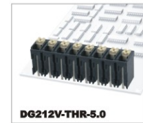
DG212V-THR-5.0 500V/17.5A 0.2-1.5mm 2 300V/12A 28-14AWG Poles 2P-24P
