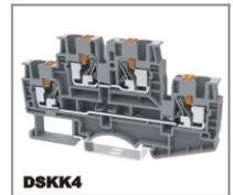
DSKK4 CE 500V/32A 0.2-6mm 2 UL 300V/28A 24-10AWG T/W/End plate 6.2/83.5/2.2mm
