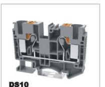
DS10 CE 1000V/57A 0.5-16mm 2 UL 600V/65A 20-8AWG T/W/End plate 10.2/67.7/1.5mm
