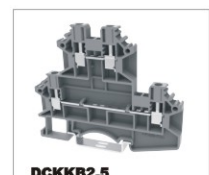
DCKKB2.5 CE 500V/24A 0.5-4mm 2 UL 300V/20A 26-12AWG T/W/End plate 5.1/76/1.5mm
