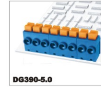
DG390-5.0 250V/13.5A 1.0mm 2 300V/8A 22-18AWG Poles 2P,3P-24P
