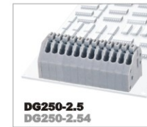
DG250-2.5 DG250-2.54 250V/2A 0.2-0.5mm 2 300V/2A 24-20AWG Poles 1P-XXP
