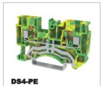
DS4-PE CE — 0.2-6mm 2 UL — 24-10AWG T/W/End plate 6.2/56/1.5mm
