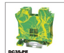
DC35-PE CE — 2.5-50mm 2 UL — 14-1/0AWG T/W/End plate 16/55.4/-mm
