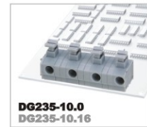
DG235-10.0 DG235-10.16 750V/15A 0.2-2.5 SOL 300V/5A 20-18AWG Poles 1P-XXP
