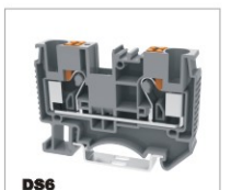
DS6 CE 1000V/41A 0.5-10mm 2 UL 600V/50A 20-8AWG T/W/End plate 8.2/57.7/1.5mm
