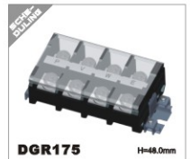
DGR175 H=48.0mm IEC 800V/175A 70mm 2 UL 600V/175A 20-2/0AWG Poles 1P-XXP
