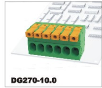
DG270-10.0 1000V/76A 0.75-16mm 2 300V/66A 24-4AWG Poles 1P-XXP
