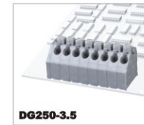
DG250-3.5 450V/5A 0.2-0.75mm 2 300V/8A 22-16AWG Poles 1P-XXP
