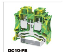
DC10-PE CE — 0.5-16mm 2 UL — 20-6AWG T/W/End plate 10/43.9/1.5mm
