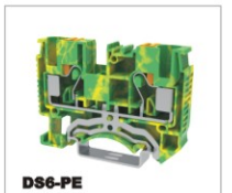
DS6-PE CE — 0.5-10mm 2 UL — 20-8AWG T/W/End plate 8.2/57.7/1.5mm
