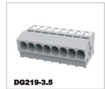
DG219-3.5 320V/17.5A(III/2) 0.2-1.5mm 2 300V/10A 24-16AWG Poles 2P-XXP
