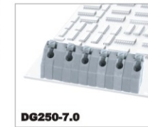
DG250-7.0 450V/5A 0.2-0.75mm 2 300V/8A 22-16AWG Poles 1P-XXP
