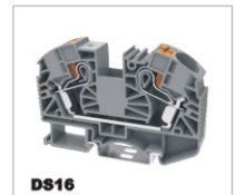
DS16 CE 1000V/76A 0.5-25mm 2 UL 600V/85A 20-4AWG T/W/End plate 12.2/75.4/2.2mm
