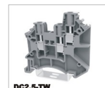
DC2.5-TW CE 1000V/24A 0.2-4mm 2 UL 600V/20A 22-12AWG T/W/End plate 5.1/48.7/1.5mm
