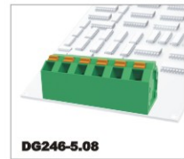
DG246-5.08 320V/9A 0.2-1.5mm 2 300V/10A 24-16AWG Poles 2P-24P
