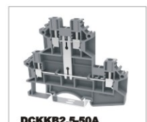
DCKKB2.5-50A CE 500V/24A 0.5-4mm 2 UL 300V/20A 26-12AWG T/W/End plate 5.1/76/1.5mm
