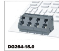
DG264-15.0 630V/76A 0.2-16mm 2 300V/66A 24-6AWG Poles 1P-XXP
