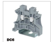
DC6 CE 1000V/41A 0.2-10mm 2 UL 600V/50A 22-8AWG T/W/End plate 8.0/45.0/1.5mm
