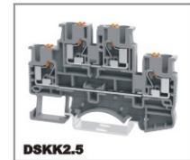
DSKK2.5 CE 500V/22A 0.2-4mm 2 UL 300V/20A 26-12AWG T/W/End plate 5.2/68.2/2.2mm
