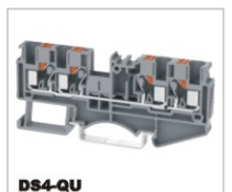
DS4-QU CE 800V/32A 0.2-6mm 2 UL 600V/30A 24-10AWG T/W/End plate 6.2/77/2.2mm
