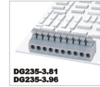
DG235-3.81 DG235-3.96 250V/10A 1.5mm 2 300V/5A 20-18AWG Poles 1P-XXP
