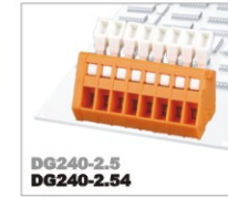
DG240-2.5 DG240-2.54 130V/6A 0.2-0.5mm 2 150V/4A 28-20AWG Poles 1P-XXP
