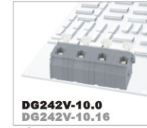
DG242V-10.0 DG242V-10.16 1000V/17A 0.2-2.5mm 2 300V/15A 28-12AWG Poles 1P-XXP
