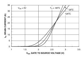
Figure 5. Transfer Characteristics.
