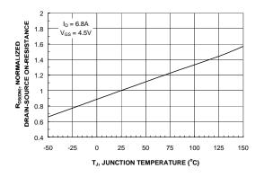
Figure 3. On-Resistance Variation withTemperature.
