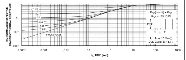
Figure 11. Transient Thermal Response Curve.
