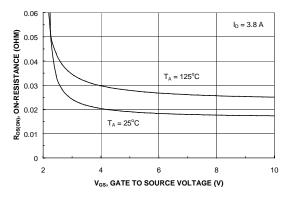
Figure 4. On-Resistance Variation with Gate-to-Source Voltage.
