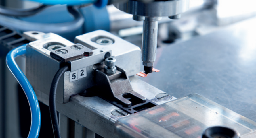
Components are comprehensively tested, measured and calibrated before packing in standard tapes and reels
