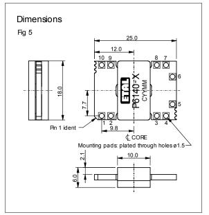
Dimensions shown are in millimetres. Terminal finish is 0.1µm max gold (Au) over nickel (Ni).
