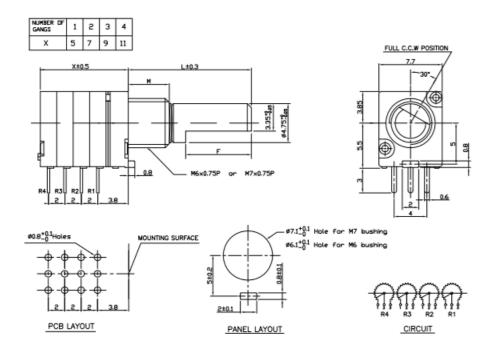
P08xS - POTENTIOMETER WITH ROTARY SWITCH MODULE
