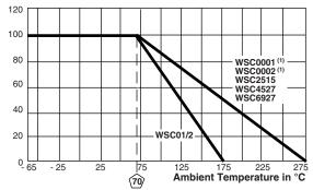
Note <sup>(1)</sup> As of 1/1/2010, WSC0001 and WSC0002 will be molded with thermoplastic and have the higher 275 °C temperature derating.
