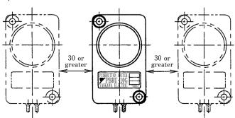
There must be 30mm or greater separation between the switch unit and other magnetic materials.
