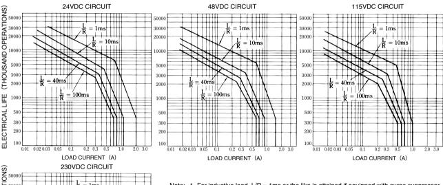
Note: 1. For inductive load, L/R = 1ms or the like is attained if equipped with surge suppressor.
