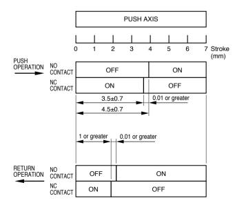
Note:Operate the plunger within the speed that the plunger can follow. (Do not release the plunger rapidly.)
