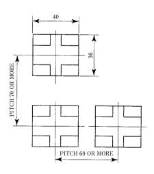
Refer to the dimensions specified below for proper mounting and separation from other magnetic materials. Units mounted closer together than specified may affect operations and result in unsatisfactory performance.
