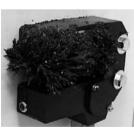
Adhesion of iron particles (60g) (If iron particles are adhered as shown in this picture, influence is only a little bit.)
