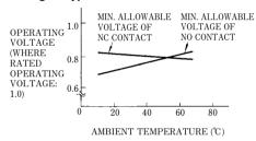
Note: Minimum allowable voltage under no load.
