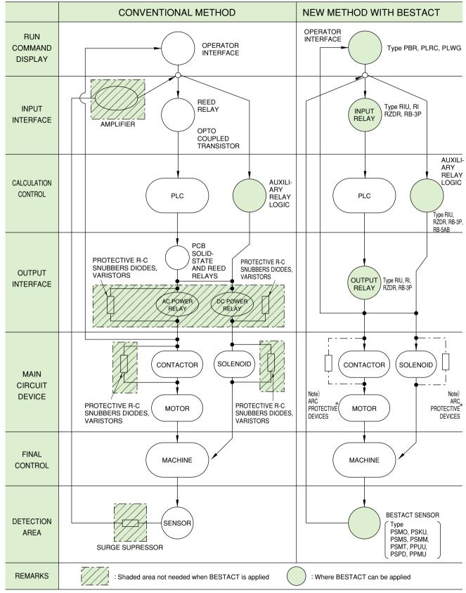
Note: \*Normally, arc protective circuitry is not needed. However, if applied, extremely long life can be obtained.
