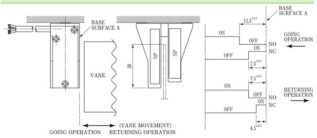
Recommended vane material: SPCC&SPHC (Magnetic material), Thickness: 1.2mm, width 50mm or greater Recommended vane inserted depth: 39mm or greater
