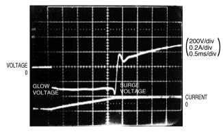
Breaking Waveform of Bestact
