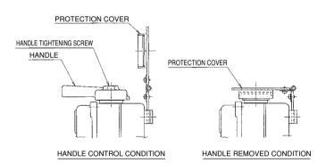
Note: 1. Control the handle with the protection cover opened up.
