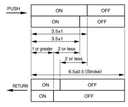
Note:Operate the plunger within the speed that the plunger can follow. (Do not release the plunger rapidly.)
