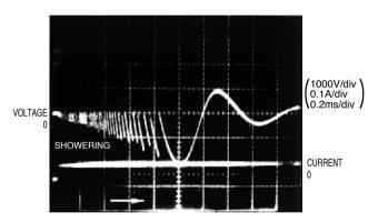
Breaking Waveform of Conventional Relay
