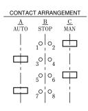
Note: when the switch is used in a DC circuit, connect odd number to +, and even number to  $\bigcirc$ .
