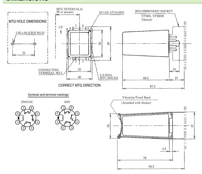
Note: 1. Mount a vibration proof band to protect relays from vibration and shock during transportation.
