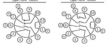
$<sup>\</sup>cdot$  Use coils and contacts according to the above polarity.
