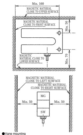
Vanes must be mounted securely so they will not contact the switches or be bent by permanent magnets incorporated in the switches.
