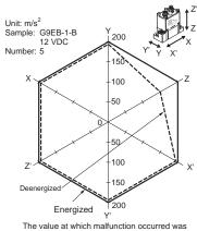
measured after applying shock to the test piece 3 times each in 6 directions along 3 axes.
