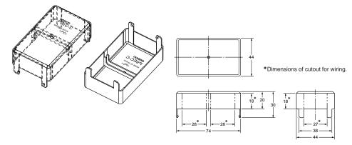
**Note:** Be sure to remove the cutouts for wiring that are located in the wiring outlet direction before installing the Terminal Cover.
