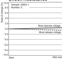
Characteristics were measured after applying a shock of 490 m $^2$ /s to the test piece 3 times each in 6 directions along 3 axes. The percentage rate of change is the average value for all of the samples.
