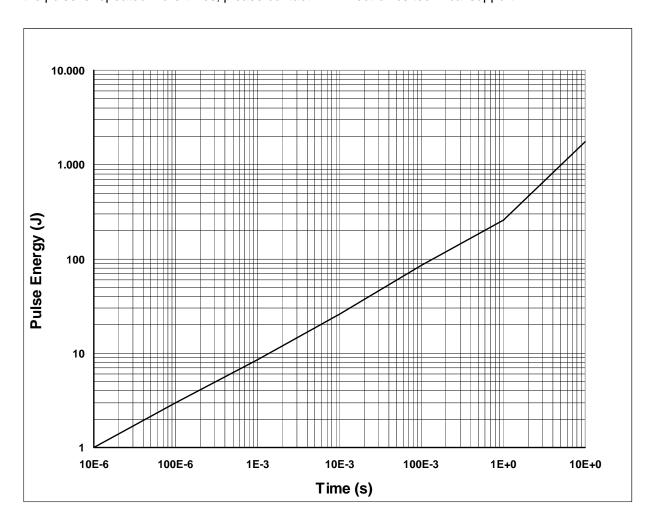
The maximum load capability for application between 10µs and 10s is indicated by the line on the graph below (Maximum heatsink temperature: 70°C).
