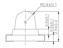
For reflow soldering (propose)
