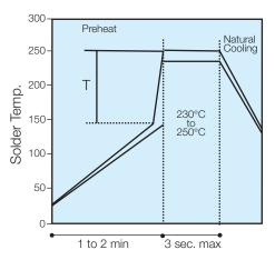
(Preheat chips before soldering) T/maximum 150°C
