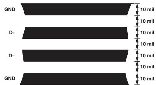
Figure 7. Arrangement of Signal Tracks
