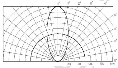
Relative Radiant Intensity vs .Angular Displacement
