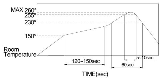
■ The condition mentioned above is the temperature on the Cu foil of the PCB surface. There are cases where board's temperature greatly differs from switch's surface be used not to allow switch's surface temperature to exceed 260°C.
