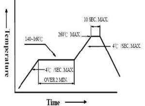
DIP soldering(Wave Soldering) : Preheating : 120°C ~150°C → within 120~180sec Operation heating : 245°C±5°C within 5 sec 260°C (Max).
