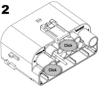
Insert contact until an audible "Click" is heard or felt. Pull slightly on wire to ensure full seating. If resistance is felt prior to full seating, refer to Section "D" to verify connector TPA is in pre-lock position.
