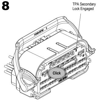
After all desired contacts are inserted, engage the TPA secondary lock. A physical resistance to fully engaging TPA indicates contacts are not fully inserted. Go back to Step 1. When an audible "Click" is heard, TPA secondary lock is in final position.
