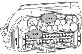
Insert contact until an audible "Click" is heard or felt. Pull slightly on wire to ensure full seating. If resistance is felt prior to full seating, refer to Section "C" to verify connector TPA is in the pre-lock position.
