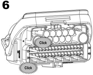
Insert contact until an audible "Click" is heard or felt. Pull slightly on wire to ensure full seating.
