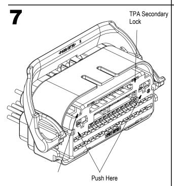
Push to activate TPA secondary lock from pre-set (out) position to fully engage.
