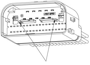
Pull TPA posts with pliers to remove TPA and alignment plate simultaneously
