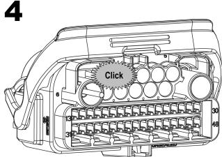
Insert contact until an audible "Click" is heard or felt. Pull slightly on wire to ensure full seating.
