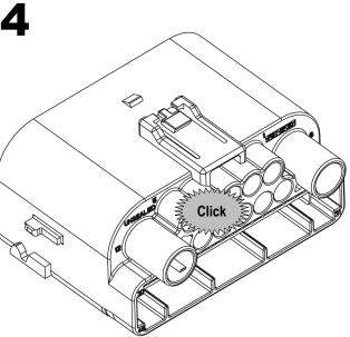
Insert contact until an audible "Click" is heard or felt. Pull slightly on wire to ensure full seating.
