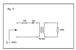
At the expense of a small loss, (approximately 1.5dBV) the circuit in fig. 3 provides an impedance exceeding  $40k\Omega$ , 200Hz-4.3kHz, and frequency response flatness within  $\pm 0.25dB$  over the same band.
