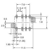
**Terminal Arrangement and Internal Connections** (Top View)
