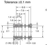
**Terminal Arrangement and Internal Connections** (Top View)
