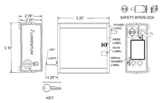
Fig. 10- Small Model 1200 Series Power Supply Dimensions. 1201-xx, 1202-xx, 1205-xx, 1206-xx, 1207-xx, 1208-xx
