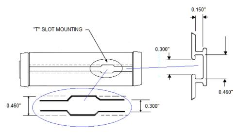
Figure 6: Model 1500 Series Bottom Plate Slot Mount
