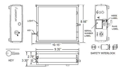
Fig. 11- Large Model 1200 Series Power Supply Dimensions. 1216-xx, 1218-xx
