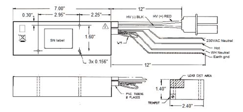
Figure 14- Module 380T Series Power Supply Dimensions
