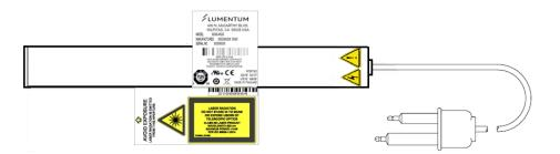
Figure 1: Placement of Safety Labels on 1100 Lasers
