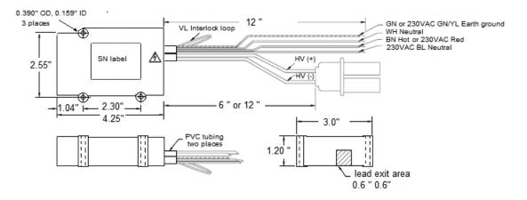
Figure 13- Module 314T Series Power Supply Dimensions
