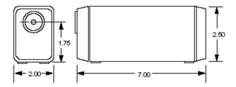
Figure 5: Model 1500 Series Laser (dimensions in inches)
