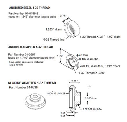
Figure 4: Model 1100 Series Accessory Bezels
