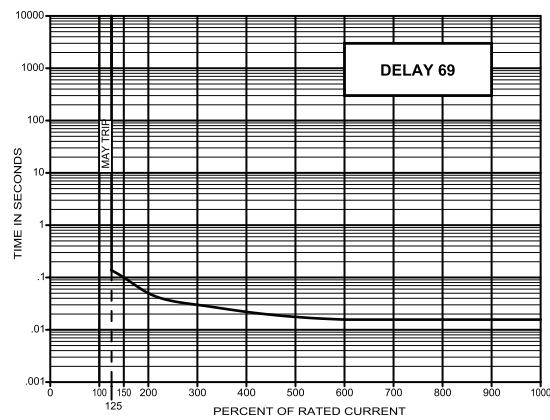
**400Hz, DC, 50/60Hz Delay Curves (typ)**
