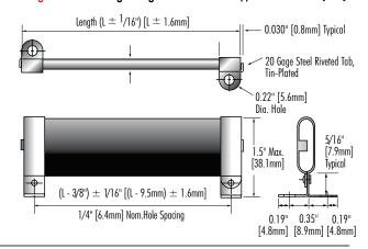
Figure 5. With Low Profile Axial Tabs (H1)
