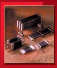
Series 500SP Non-Inductive Bulk Ceramic Slab Resistors Series 500SP Non-Inductive Bulk Ceramic Slab Resistors provide high power and energy dissipation in a compact size. Proprietary bulk ceramic "SP" material is used in a simple, efficient design that permits energy to be uniformly absorbed throughout the resistor body, thereby avoiding failure in a peripheral film or wire.
