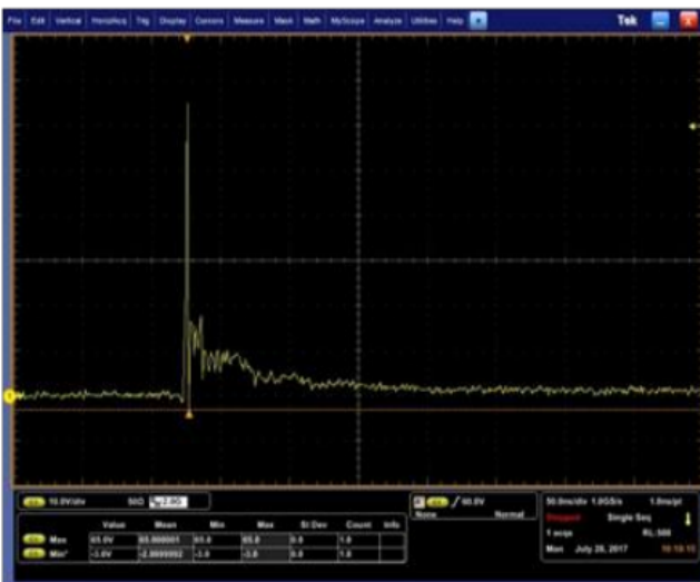
Figure 1. ESD Clamping Voltage Screenshot Positive 8 kV Contact per IEC61000-4-2
