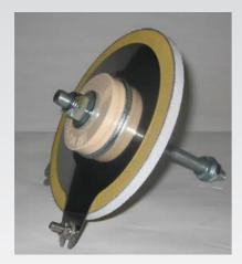
In some applications of high impedance relays, a non-linear Metrosil resistor is required to limit the current transformer (CT) secondary voltage to a safe level during maximum internal fault conditions.
