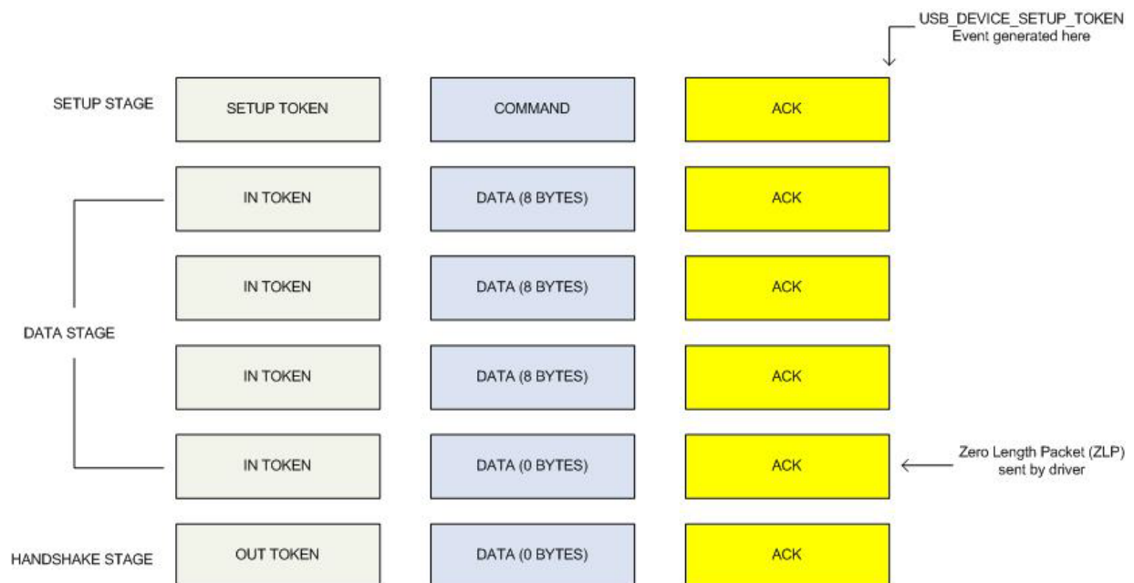
Figure 6: Multi Transaction Control Read Transfer with ZLP (Data size is 24 bytes and maximum endpoint size is 8 bytes)
