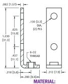
.062 (1.57) thick Steel, Nickel Plate
