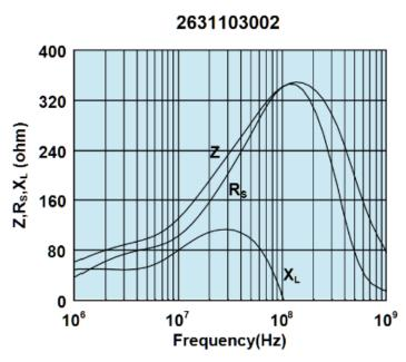
Impedance, reactance, and resistance vs. frequency.
