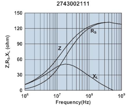
Impedance, reactance, and resistance vs. frequency.
