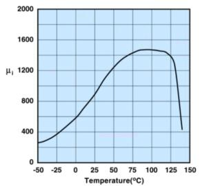
Measured on a 17/10/6mm toroid at 100kHz.
