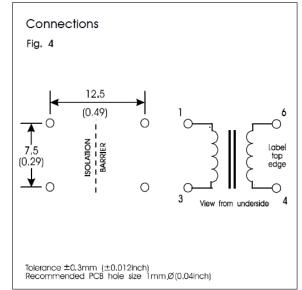
Dimensions shown are in millimetres (inches). Geometric centres of outline and pin grid coincide within a tolerance circle of 0.6mmØ. Windings may be used interchangeably as primary or secondary.
