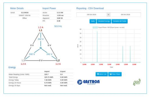
In this view the user is able to interrogate information such as line to line voltages, reactive power, power factor and mains frequency, to allow them to diagnose issues with individual power supplies in the network.
