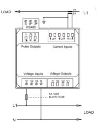
Single phase two wires (No Voltage Output on SMART X96-5E Model)
