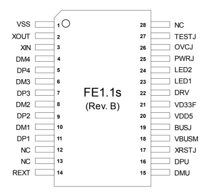
Fig. 2: 28-Pin SSOP Pin Assignment
