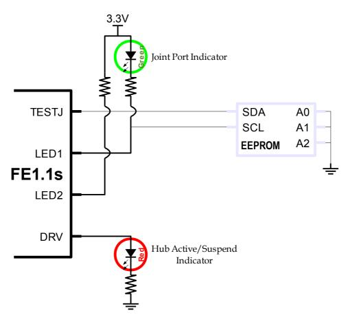
Fig. 5: Joint Port Indicator Configuration
