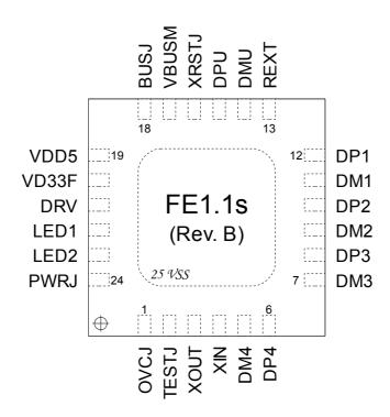
Fig. 3: 24-Pin WQFN Pin Assignment
