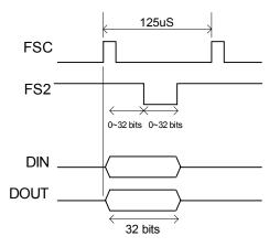
DOUT is open-collector, it should be pulled high with an external pull-up resistor. Outside the 32 bit data transfer window, DOUT can either be set to float or DOUT pins can be forced to drive low. This option allows some peripherals to activate the data clock.
