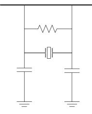
The recommended resister value is 1M ohm, capacitors should be 10pF. The crystal should be placed close to the Tiger320 and good layout practice followed.
