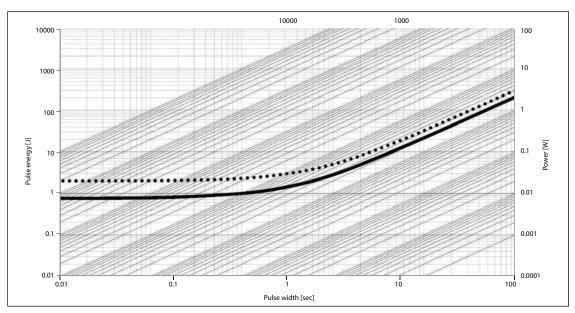
In this graph the max. & min. curve are shown as ••• and — for all resistance values, the area between the max. & min. curve is applicable. In case the Design Engineer requires a specific graph of a particular component it can be supplied on request.
