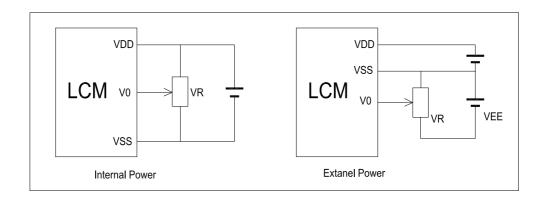
$V_{DD^{\sim}}V_0$ : LCD Driving voltage
