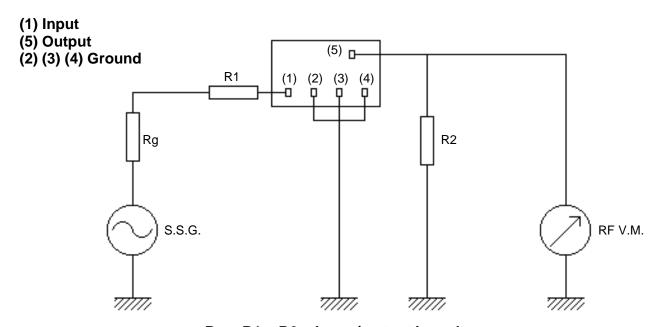
Rg + R1 = R2 = Input / output impedance
