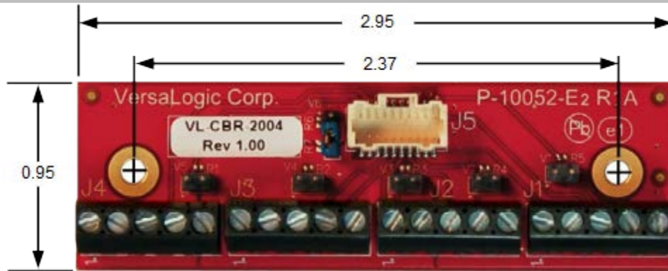
Figure 30. CBR-2004B/CBR-2005 Dimensions and Mounting Holes
