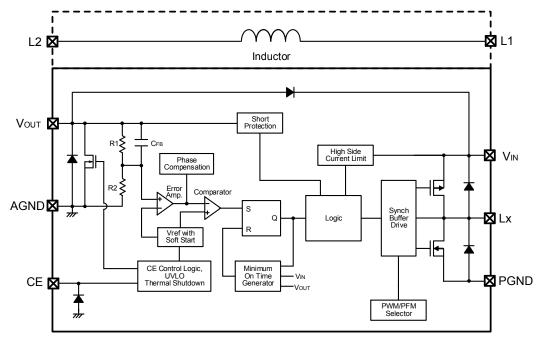
\* The XCL221 offers a fixed PWM control, a Control Logic of PWM/PFM Selector is fixed at "PWM" internally.
