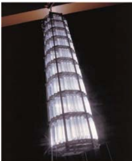
Artificial quartz crystal drawn from an autoclave
